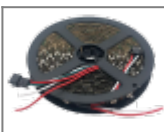
WS28xx: addressable RGB LEDs
